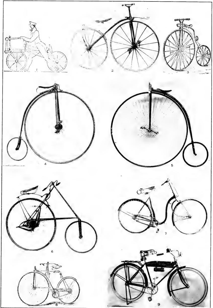
1, Draisine or hobby horse, 1818; 2, Lallement velocipede, 1869; 3, J. K. Starley "Ariel", 1873; 4, Columbia "Ordinary", 1885; 5, Humber racing "Ordinary", 1885; 6, American "Star", 1885; 7, Lady's "Victoria" 1887; 8, Starley and Sutton "Rover" 1885; 9, Snyder "De Luxe", 1928.
